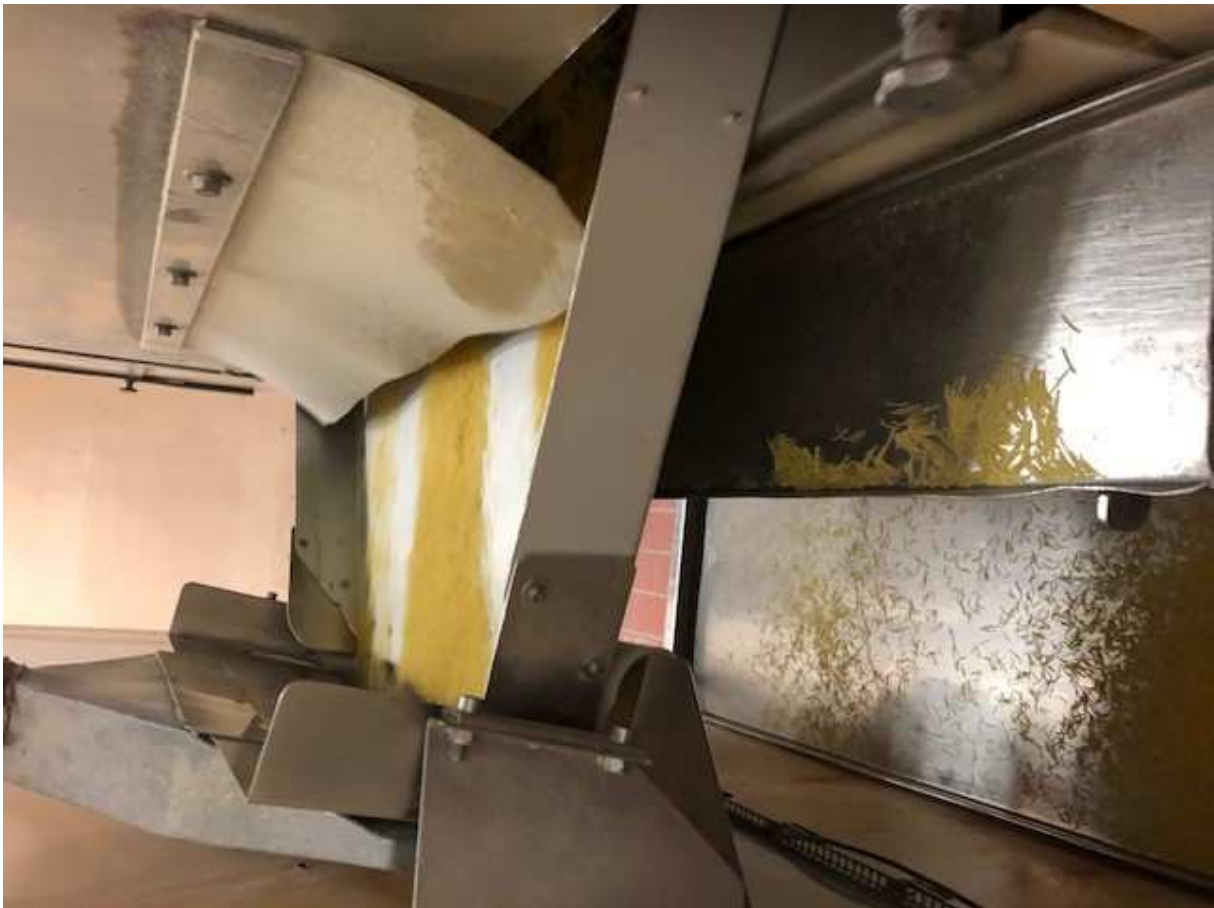
Discharge Bühler Shaker Pre Dryer – Intake Drum Dryer TROA
